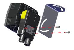
Align the holes on the mounting surface with the mounting holes on the reader. With the reader in right-angle position, only the back mounting holes can be used.
