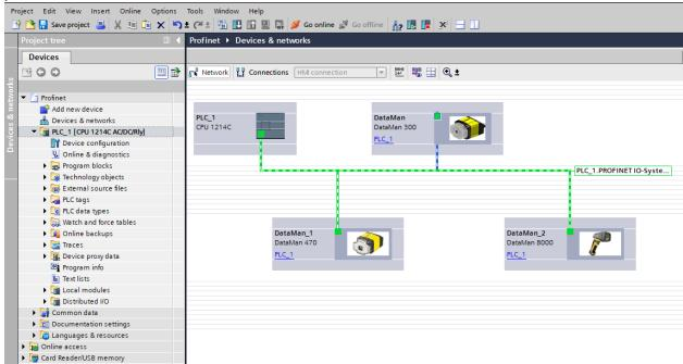
12. By default, the SIMATIC software maps the User Data and Result Data Modules to offset 256. This is outside of the default process image area size of 128. That is, data in these modules are inaccessible by some SFCs such as BLKMOV. As a solution, either remap the modules to lower offsets within the process image area or expand the process image area to include these modules.
