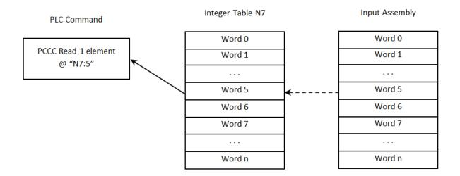
The decode ResultData begins at byte offset 16 (counting from 0) of the Input Assembly. To read the first 4 bytes of result data, issue the following PLC command:
