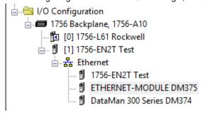
7. When the Generic Module is added to the I/O tree, RSLogix 5000 creates tags that map to the DataMan reader Input and Output Data (that is, the Input and Output Assembly Objects in the DataMan Reader). You can find these tags under the "Controller Tags" node of the project tree.
