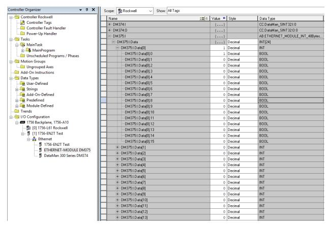
Output Assembly "Trigger": Bit 1 of word 0 of the Output Assembly. From the Output tag array for the DataMan select bit 1 of word 0.
