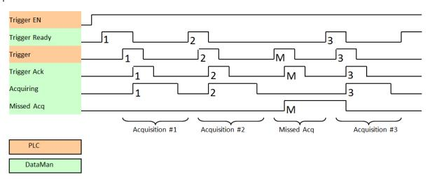
To force a reset of the trigger mechanism, set the *TriggerEnable* to False until *TriggerReady* is also set to False. Then, *TriggerEnable* can be set to True to re-enable acquisition.
