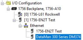
8. When the DataMan module is added to the I/O tree, RSLogix 5000 creates tags that map to the DataMan reader Input and Output Data (that is, the Input and Output Assembly Objects in the DataMan Reader). These tags can be found under the "Controller Tags" node of the project tree.
