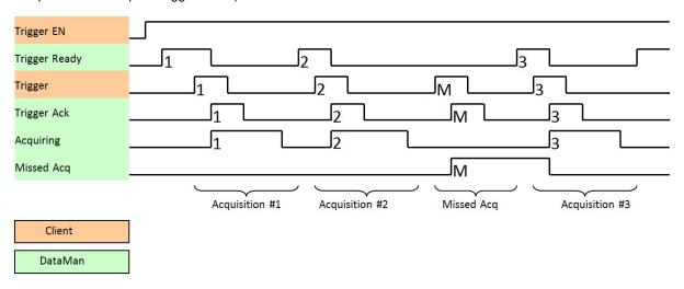
To force a reset of the trigger mechanism, set the AcqTriggerEnable attribute to False until the AcqStatusRegister is 0. Then the AcqTriggerEnable can be set to True to re-enable acquisition.
