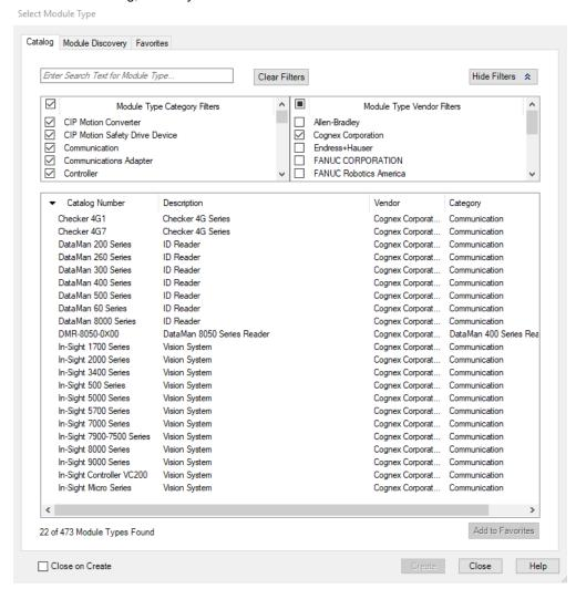
After the selection is completed, the configuration dialog for the DataMan ID Reader system is displayed. From this point on, configuration and programming are done exactly as shown in the ControlLogix section above.
