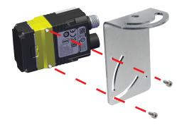
Align the holes on the mounting surface with the mounting holes on the reader. Insert the M3 screws into the mounting holes.
