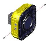
3. Slide the reader into the mounting bracket through the central slot.
