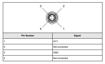
**CAUTION**: Do not use the LIGHT connector to power the integrated light externally.
