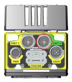
2. Connect the RJ-45 connector of the Ethernet cable to a switch, router, or PC.
