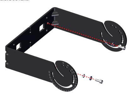
2. Insert the rotation axis screws without fully tightening them.
