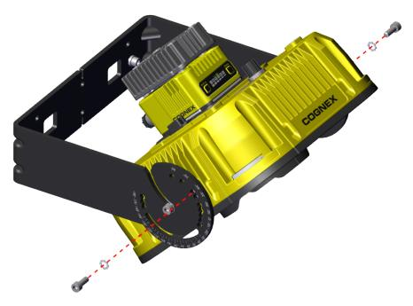
5. Tighten the mounting screws.
