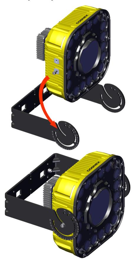
4. Apply the chosen rotation angle by inserting a screw into one of the preset holes or to the sliding slot on the mounting bracket.
