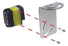
Align the holes on the mounting surface with the mounting holes on the reader. Insert the M3 screws into the mounting holes.
