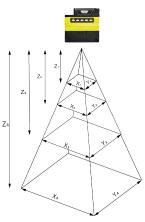
The following table shows the Field of View (FoV) widths of the 6.2 mm lens focused to 190 mm at various distances.
