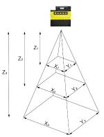
The following tables show the Field of View (FoV) widths of the  $6.2\ mm$  lens focused to  $105\ mm$  at various distances.
