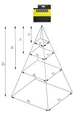
The following tables list the Field of View (FoV) widths of the 16 mm lens at various distances:
