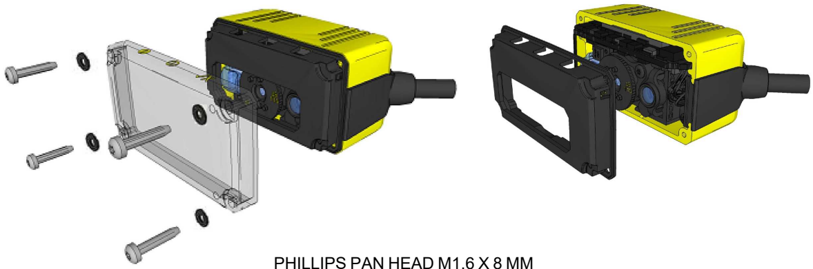
PHILLIPS PAN HEAD M1.6 X 8 MM
