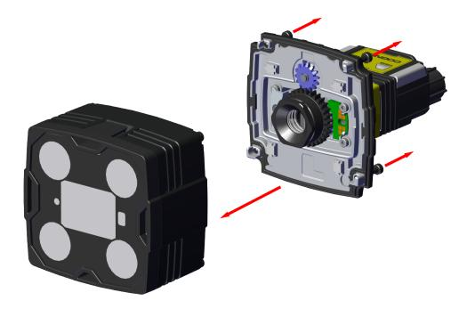
2. Unscrew the two screws from the housing using a 1.5 mm hex key.
