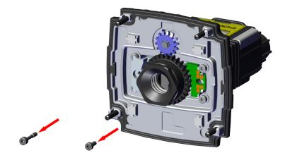
0 **Note**: Start disassembling with unscrewing the M2 x 12 mm HSH screw on the left side. Continue unscrewing with the M2 x 5 mm HSH screw on the right side.
