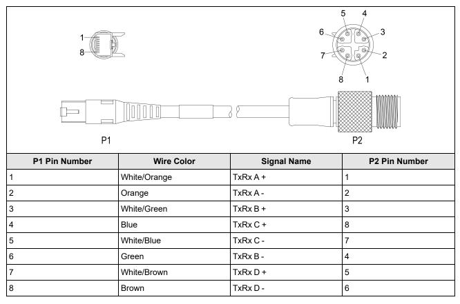
**CAUTION**: The Ethernet cable shield has to be grounded at the far end. Whatever this cable is plugged into (typically a switch or router) should have a grounded Ethernet connector. A digital voltmeter has to be used to validate the grounding. If the far end device is not grounded, a ground wire should be added in compliance with local electrical codes.
