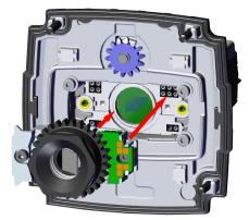
b. Tighten the M2 x 5 mm HSH screw halfway, then tighten the M2 x 12 mm HSH screw halfway as well. Continue screwing each screw incrementally, tightening them to 0.3 Nm using a torque wrench.
