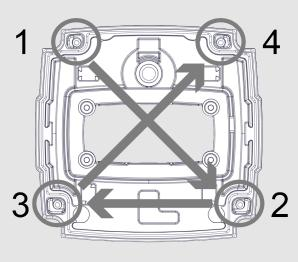
4. Screw in the four screws from the light module into the front cover.
