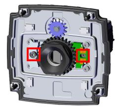
() Note: Start reassembling with the M2 x 5 mm HSH screw on the right side.
