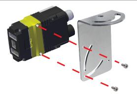
Align the holes on the mounting surface with the mounting holes on the vision system. Insert the M3X3.5 screws into the mounting holes.
