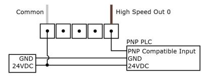
To connect the high-speed outputs to a relay, LED or similar load, connect the negative side of the load to the output and the positive side to +24VDC. When the output switches on, the negative side of the load is pulled down to less than 3 VDC, and 21 VDC appears across the load. Use a protection diode for a large inductive load, with the anode connected to the output and the cathode connected to +24 VDC.
