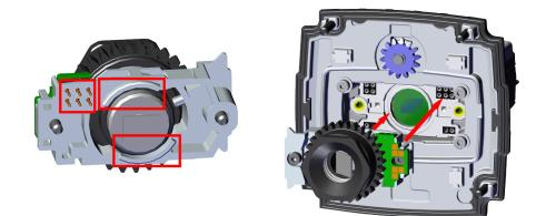
b. Tighten the M2 x 5 mm HSH screw halfway, then tighten the M2 x 12 mm HSH screw halfway as well. Continue screwing each screw incrementally, tightening them to 0.3 Nm using a torque wrench.
