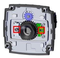
(i) Note: Start reassembling with the M2 x 5 mm HSH screw on the right side.
