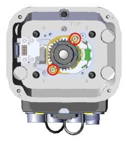
6. Replace the adapter on the sensor.
