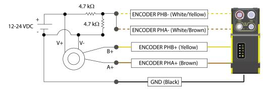
The image below shows the wiring of a differential encoder.
