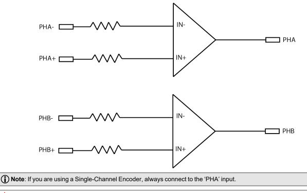
WARNING: The frequency of pulses has to remain under 1000 kHz.
