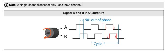
The distance per cycle is the physical distance that the conveyor system needs to travel to cause the encoder to output one full cycle. This distance can be calculated based on the dimensions of your encoder and the length of the image you want to acquire.
