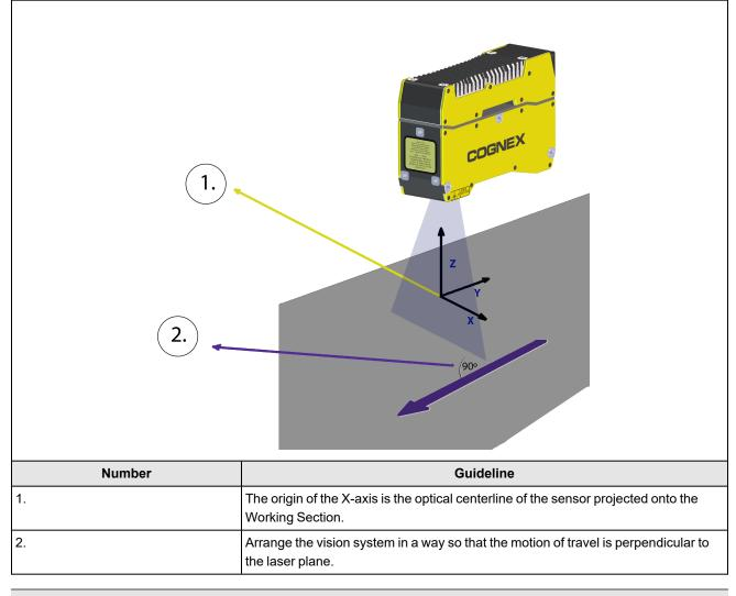
Note: The vision system can shut down above maximum operating temperature. To avoid overheating you can heatsink the vision system by attaching a 400 mm aluminum profile or surface of a thermally conductive material (for example robot mounting plate) on top of the unit.
