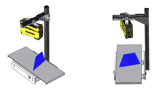
In order to generate an accurate 3D image of a scene, you have to correct the relative motion between a vision system and a motion stage in terms of Motion Direction and Motion Speed (or Encoder Resolution in case of encoder acquisition). If you do not correct Motion Direction, the scanned image can be skewed or distorted. If you do not correct Motion Speed, the scanned image can be elongated or squeezed.
