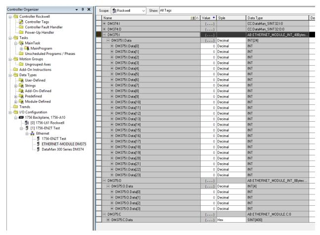
Input Assembly "ResultLength": Word 7 of the Input Assembly. From the Input tag array for the DataMan select word 7.
