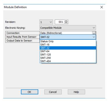
**Output Data to Sensor**: Defines the amount of data transmitted on the connection (to the DataMan). The minimum amount is the Control data only. The connection can be configured to also send user data. The amount of user data sent is defined in fixed increments (16 bytes, 32 bytes, 64 bytes, and so on). To enable User Data output, right-click the DataMan module and then go to Properties -> Change -> Output Data to Sensor.
