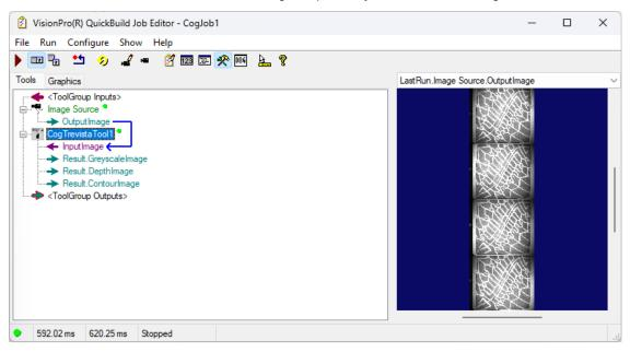
9. Open the Trevista tool edit control. The following figure shows the edit control viewing the depth image the tool generates:
