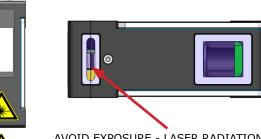
AVOID EXPOSURE - LASER RADIATION IS EMITTED FROM THIS APERTURE
