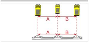
Use supplied T-nuts and screws to mount targets to rail.
