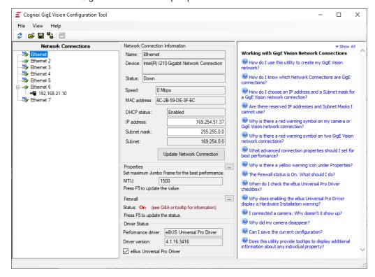
Refer to the Q&A in the far-right panel for user assistance. In addition, refer to the GigE Vision Cameras User's Guide, installed with VisionPro in the %VPRO\_ROOT%\Doc\en\HardwareManuals\GigEGuide.pdf.
