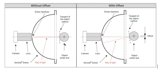
Ensure pro per camera alignment with the dome aperture (concentricity). This is best done from inside the dome. Examine the lens to check if it is concentric with the dome aperture.
