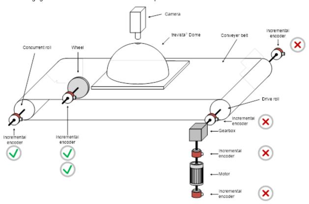
The following figures show suitable and unsuitable encoder positions for rotary motion:
