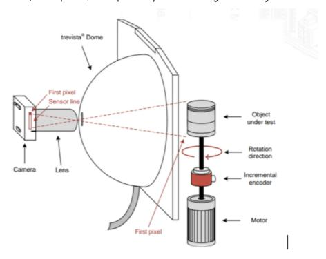
If the parts are highly reflective, the dome aperture may be visible in the image causing a dark spot in the image. Tilting the dome slightly (or the part) can prevent this. For cylindrical parts, a potential solution could be to shift the part by a small offset.
