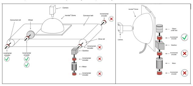
If the encoder is tracking the motion of a large object, consider whether the smallest displacement it can track matches the spatial resolution (the physical space each image pixel represents). There can be situations where this number might not be enough. In such cases, it's advisable to think about moving the encoder to a different location.
