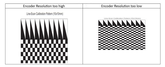
Fine-tune the Encoder Resolution value until the image appears without any noticeable distortion and the pixels appear square.
