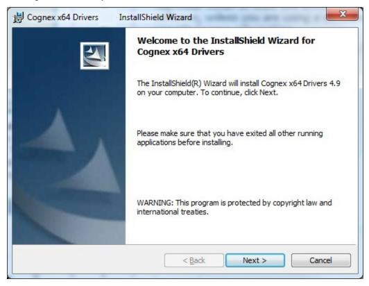
The **Cognex Drivers** utility will install the GigE Vision drivers and all the frame grabber drivers. You can, as an option, select **Custom** in the **Setup Type** dialog and pick the specific drivers you want installed. The drivers are Authenticode signed with a Cognex certificate.
