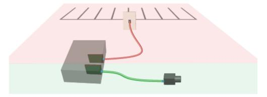
If you are using more than one camera, you can use a multi-port network adapter or a Gigabit Ethernet switch (shown):
