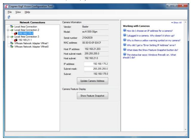
2. Enter an IP Address and a Subnet mask for the camera.
