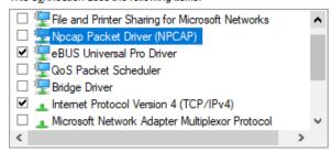
Ensure any third party Ethernet driver is either disabled on the network stack, as shown in the previous figure, or uninstalled.
