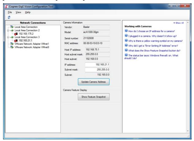
The center panel displays information about the available network connections and cameras. In most environments at least one of your **Local Area Connections** is associated with the network connection of the PC. Check with your network administrator if you are not sure which one it is.
