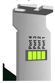
A lit LED indicates a port is supplying power over PoE. If you connect a GigE Vision camera that does not use Power over Ethernet, the LED does not light.
