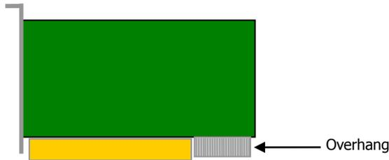
Do not confuse PCI slots with PCI Express. PCI Express is a newer high-speed serial interconnect. PCI cards cannot be placed in PCI Express slots.
