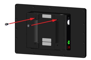
$2. \quad \text{Slide the VisionView Web panel on the table top stand so that the screws catch onto the notches in the stand}.$
